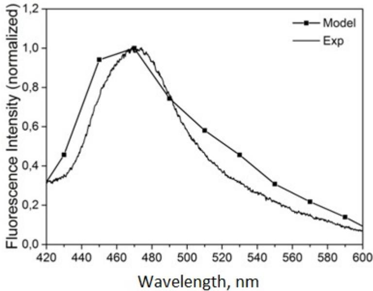
Figure 3. Comparison of experimental and model based spectra, calculated using the Monte-Carlo method. Model simulates presence of NADH and collagen.
