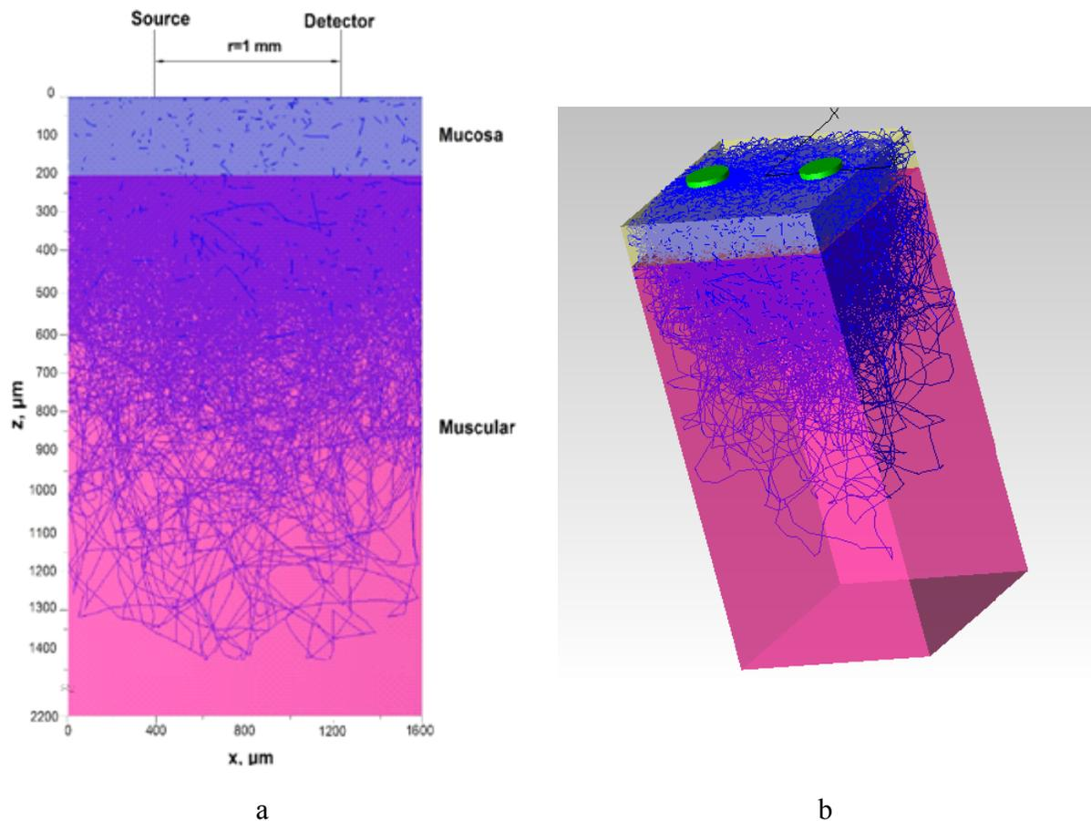
Figure 2. (a) Side view of 3D model. Source, detector and the tissue layers are labelled. The lines indicate the passage of individual photons through the tissue. Darker lines indicate the photons which are heading directly towards the visible flat surface. (b) Full 3D view of model represented in figure 2a. Source and detector are represented by green circles.
