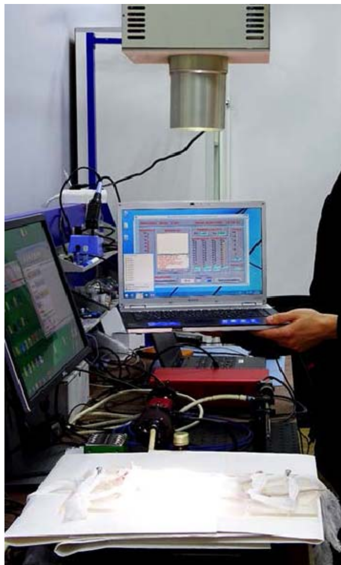
Fig 1. Installation of a color-dynamic surgical light above the operating table.
