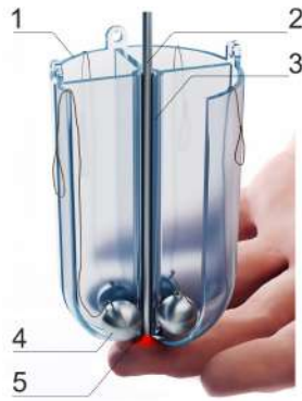
Fig. 3. 3D-printed pressure distribution tool coaxially allocated to the fibre optical probe. 1 – pressure distribution tool; 2 – fibre-optical probe 3 – central guide tube for the probe; 4 – lead weights; 5 – tip of the fibre-optical probe.
