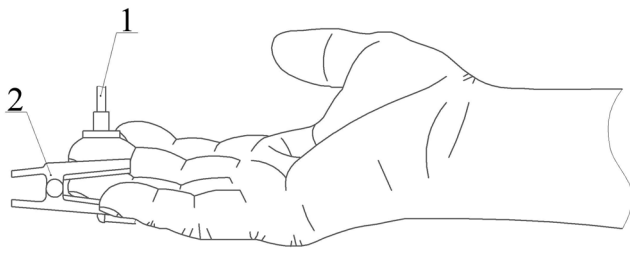
Fig. 1 Schematic presentation of the LDF probe positioning on a finger: (1) LDF probe and (2) pulseoximetry sensor.
