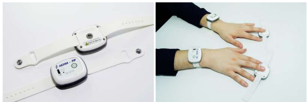
Figure 1. The appearance of the analysers (left) and the options for mounting them on the volunteer’s hands (right).
