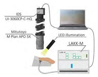
Figure 1. Scheme of the experimental setup.
