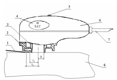
Fig. 2. The scheme of location of temperature reformer, on bio-tissue in terminal of device: 1 – connection cable of temperature reformer, 2 – temperature reformer DS1820, 3 – camera, 4 – button RAY, 5 – indicated diode of switch of laser, 6 –the body of terminal, 7 – electric cord, 8 – bio-tissue.
