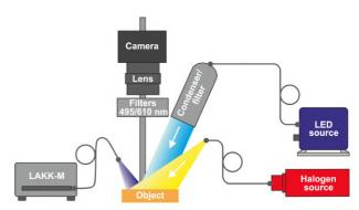
Fig. 1 The scheme of the experimental setup.
